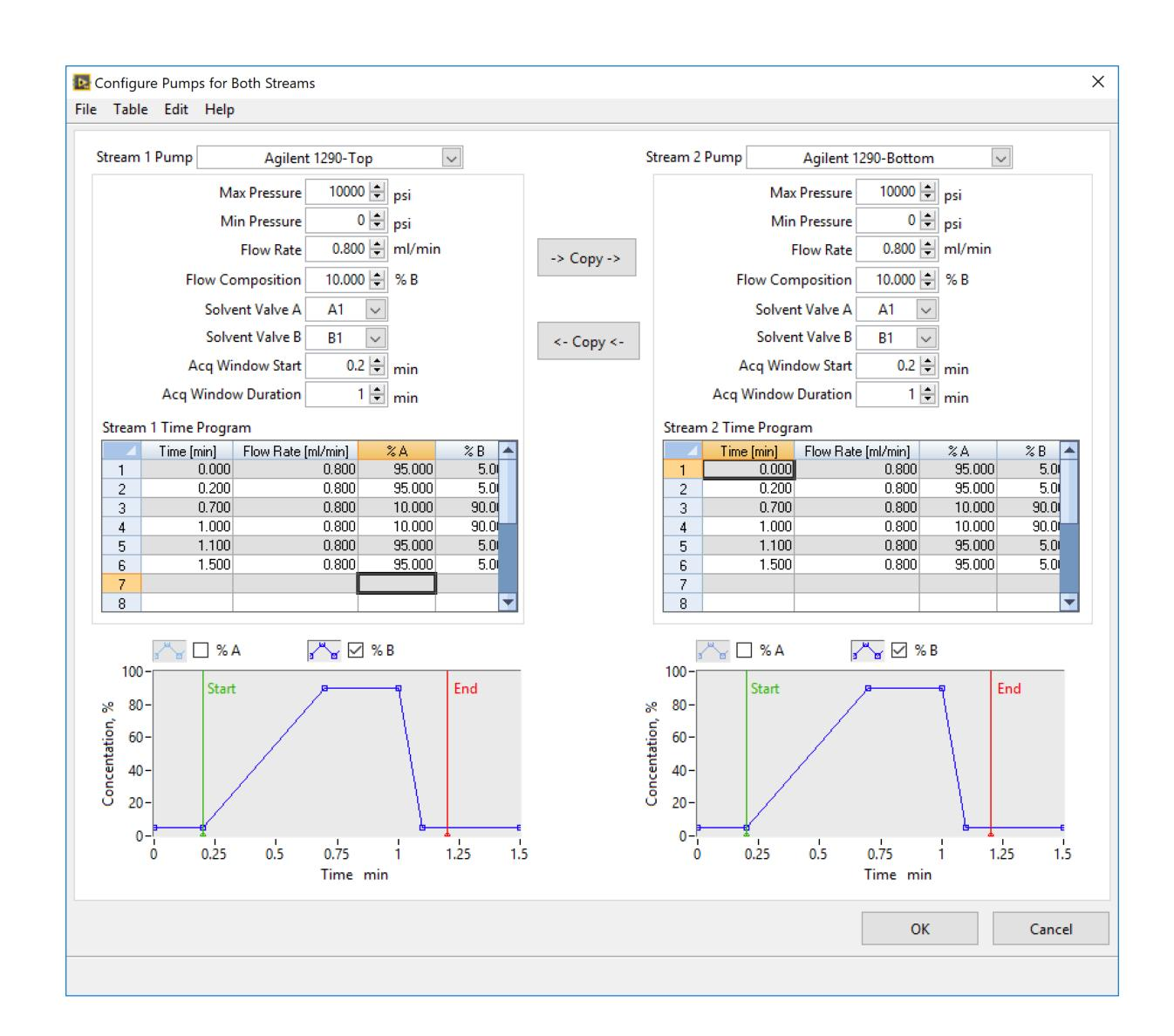
Figure 4. LC Pumps Setup. Acquisition start and duration for streams is entered in the Pump setup. Samples are run one injection per raw data file with data saved to wiff only during the specified acquisition window.
