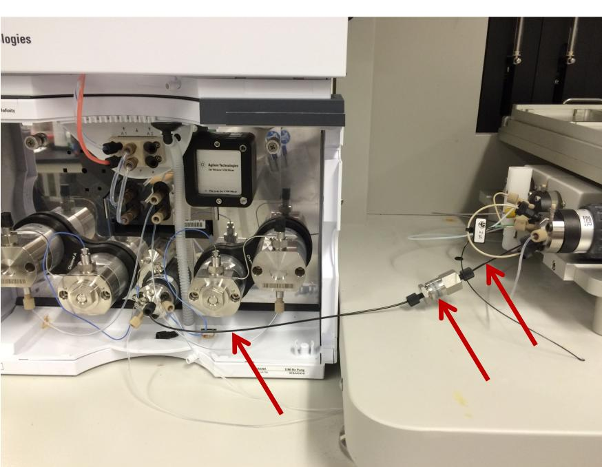
Fig 1b. To optimize the pump for microflow, low-volume PEEK tubing (0.1mm ID) and external 1µL mixer were installed using the shortest possible lengths to reach the injection port, reducing dead volume and delay time.
