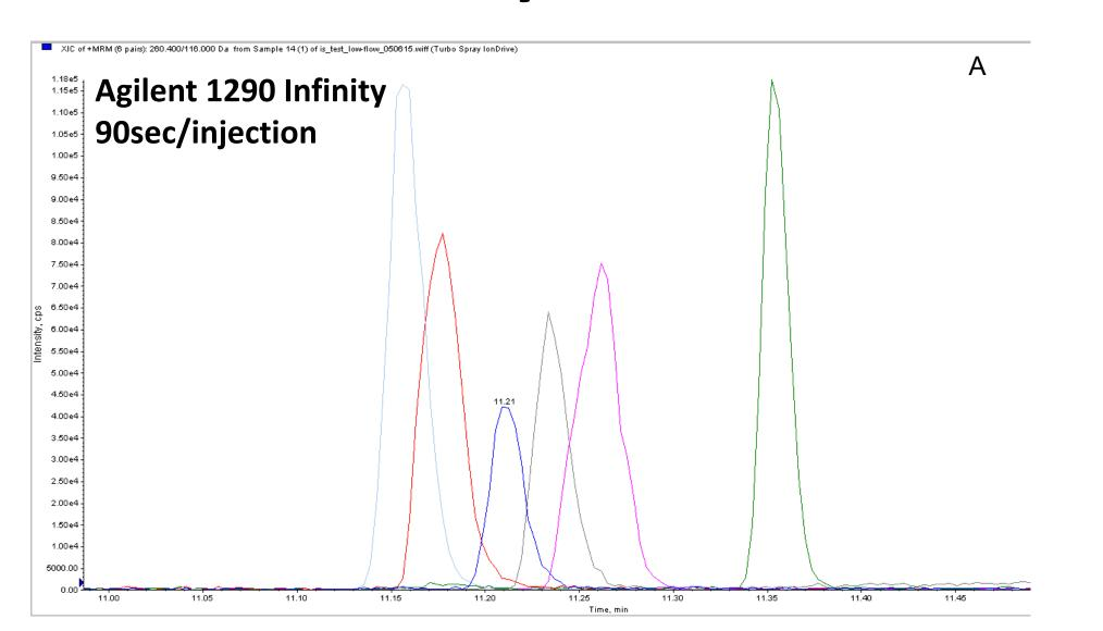
Fig 2a. 2µL injections of method development cocktail at 50µL/min (90sec/injection cycle time) using optimized Agilent 1290 Infinity UHPLC. Peak widths were ~4sec.
