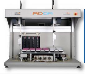
Dual-arm (dual-stream) liquidhandler-type LC/MS/MS autosampler
