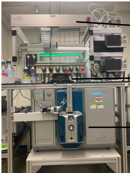
Fig2. Ultra-sensitive microflow LC-MS/MS system & components
