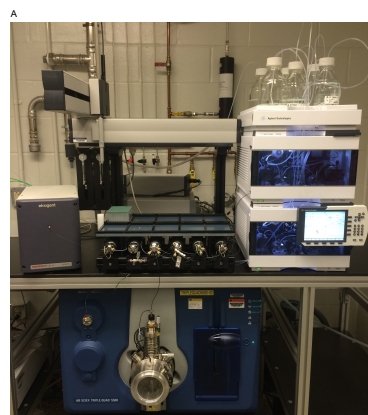
Fig 1a. The system was designed to occupy the smallest possible footprint, enabling co-location of autosampler, pumps and mass spectrometer and substantial reduction in total system volume (~5µL)
