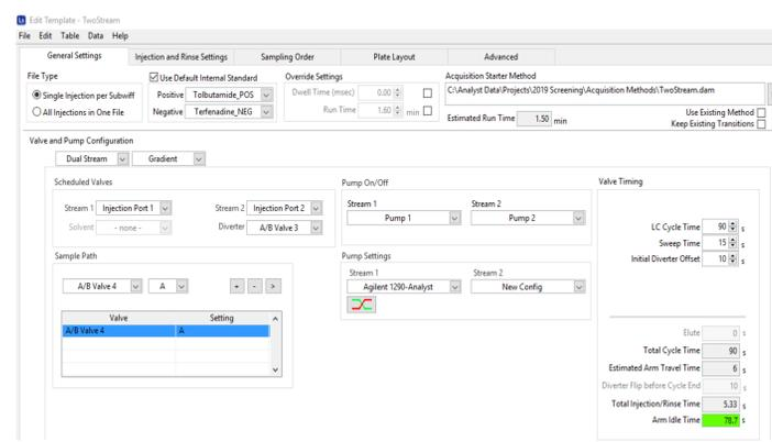
Figure 3. LeadScape Template contains File type, Valve and Pump configuration, Injection and Rinse settings, Sampling and Plate Layout, and Default mass spec acquisition method with source conditions.
