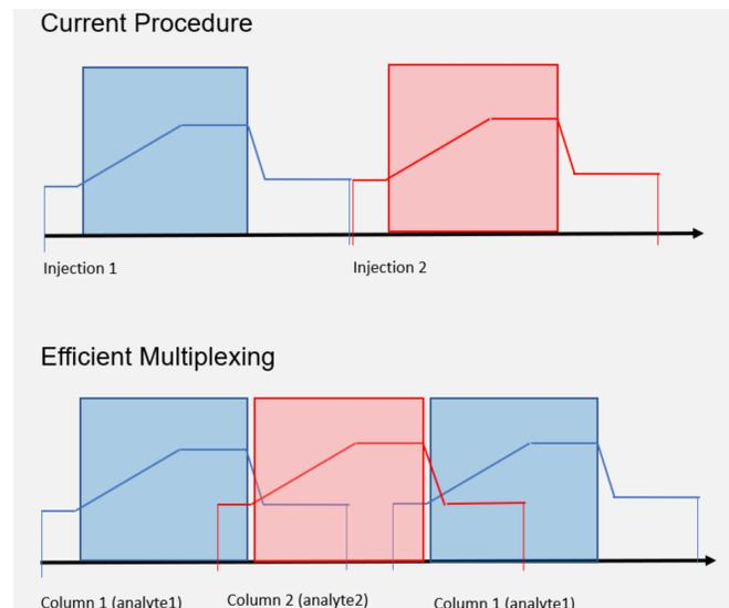
Figure 1. LS-I Efficient multiplexing utilizes equilibration time to start next injection on a separate column.
