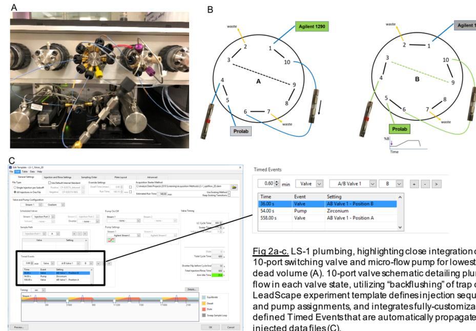
Fig 2a-c. LS-1 plumbing, highlighting close integration of injector, 10-port switching valve and micro-flow pump for lowest possible dead volume (A). 10-port valve schematic detailing plumbing and flow in each valve state, utilizing "backflushing" of trap column (B). LeadScape experiment template defines injection sequence, valve and pump assignments, and integrates fully-customizable, user-defined Timed Events that are automatically propagated for multi-injected data files (C).
