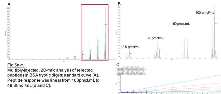
Fig 5a-c. Multiply-injected, 2D-mflc analysis of selected peptides in BSA tryptic digest standard curve (A). Peptide response was linear from 100pmol/mL to 48.8fmol/mL (B and C).
