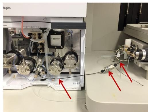
**Fig 1b.** To optimize the pump for micro-flow, low-volume PEEK tubing (0.1mm ID) and external 1µL mixer were installed using the shortest possible lengths to reach the injection port, reducing dead volume and delay time.
