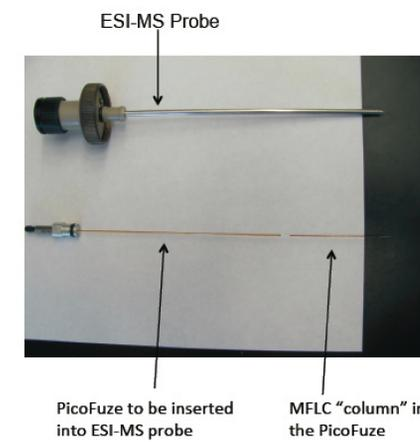
**Fig 4b.** A modified SCIEX probe houses the PicoFuze assembly. Dimensions were 50x0.2mm, tip size 20µ, and packing material was Reprisil-PUR C18, 3µ, 120A.
