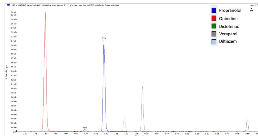
**Fig 4a.** Single injection of cocktail on PicoFuze probe using Eksigent ExpressHT pump, 3min/injection at 12µL/min. Gradient was linear from 0 to 90%B. Peak widths were ~2sec.
