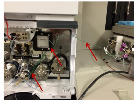
**Fig 1a.** When configured for HPLC/UHPLC, The Agilent 1290 Infinity has extensive dead volume (arrows) within transfer tubing and 35µL JetWeaver mixer. This makes high-performance micro-flow LC difficult. Efforts were focused on modifying setup and plumbing to accommodate high-performance micro-flow LC/MS/MS.
