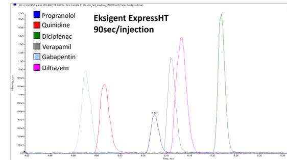
**Fig 2b.** 2µL injections of method development cocktail at 50µL/min (90sec/injection cycle time) using Eksigent micro-flow LC system. Peak widths were ~3sec.
