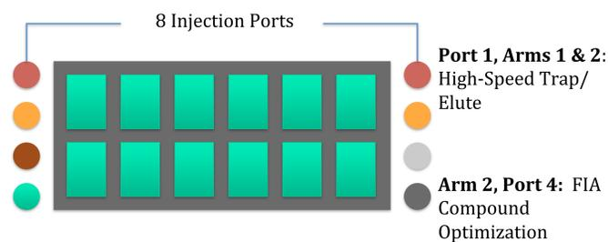
Figure 2. ADDA Injection Port configuration for experiment
