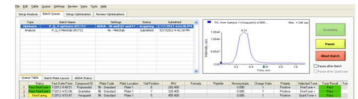
Figure 6. Queue during Optimization, performing the FineTune operation having passed QuickTune.
