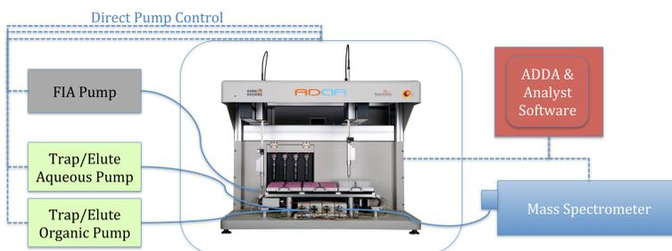
Figure 1: Simultaneous setup of the FIA and Trap/Elute analysis.
