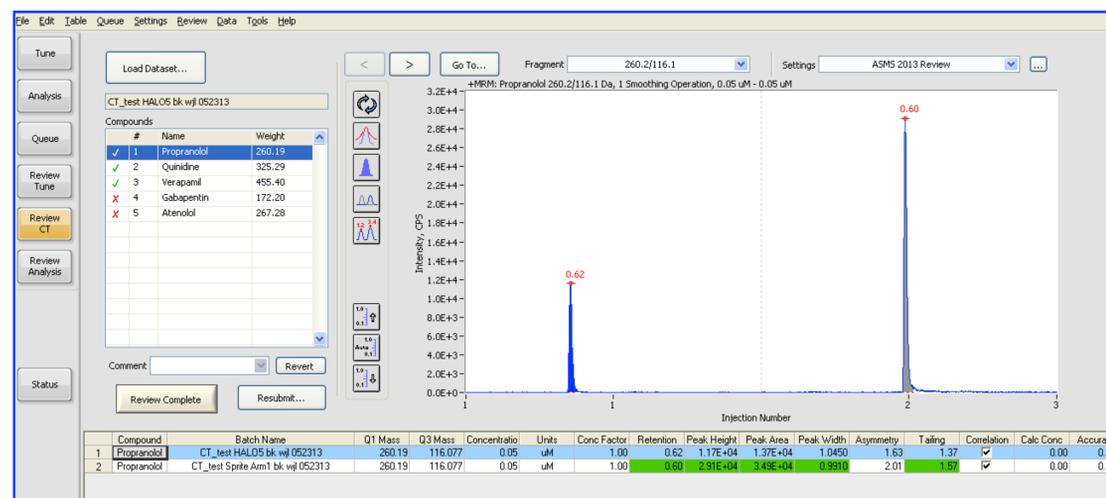
Figure 4: ChromaTune™ quality visualization panel of each compound set (with two ChromaTune™ setups selected). The peak intensity, along with peak shape and tailing are measured against set criteria. Results are shown in the chart under the peaks. As the user scrolls down the compound list, each set of ChromaTune™ results is updated in the graph, and on the chart. In this way, results from multiple runs can be compared using the same review criteria.
