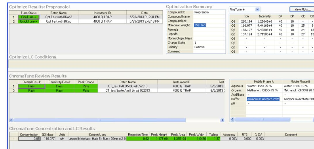
Figure 5: The Compound Optimization panel shows a summary of the full results of the compound optimization, along with a summary of the ChromaTune™ Review results run on that compound, each with peak characteristics shown in the lowest chart. LC conditions for each run are shown as well.
